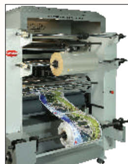
Reel Rewinding Unit
